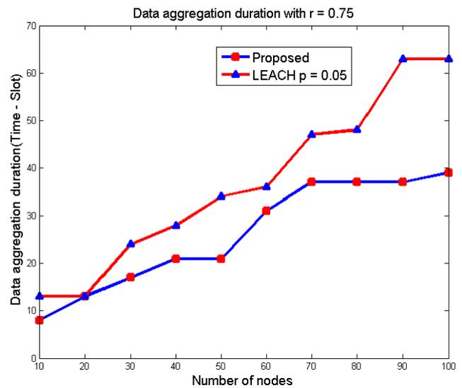
Figure 6 Total Data Aggregation Time at CR=0.75
